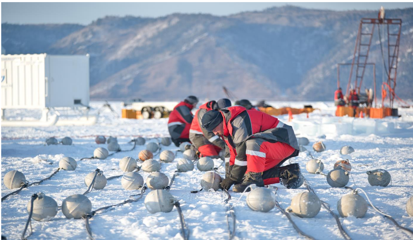
Fig. 12. Assembling the Baikal-GVD installation cluster garland
